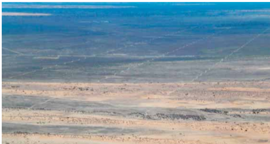
Figure 27. 3D seismic lines at Cooper Basin, South Australia – note undulating survey lines, rather than straight lines [Source: Committee site visit, 3 September 2014]
