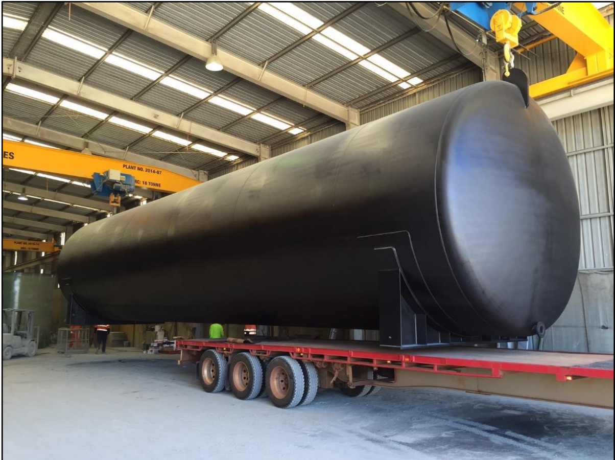
1,250 bbl storage tank under construction
