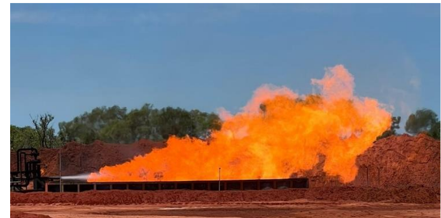
Rafael 1 flow to flare pit
