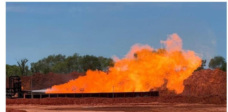
Rafael 1 flow to flare pit
