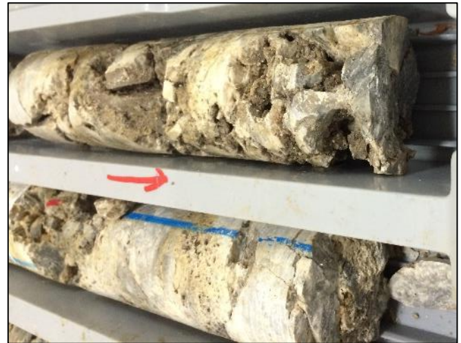
Well developed vugular porosity in the Ungani Dolomite in the Ungani Far West 1 well
