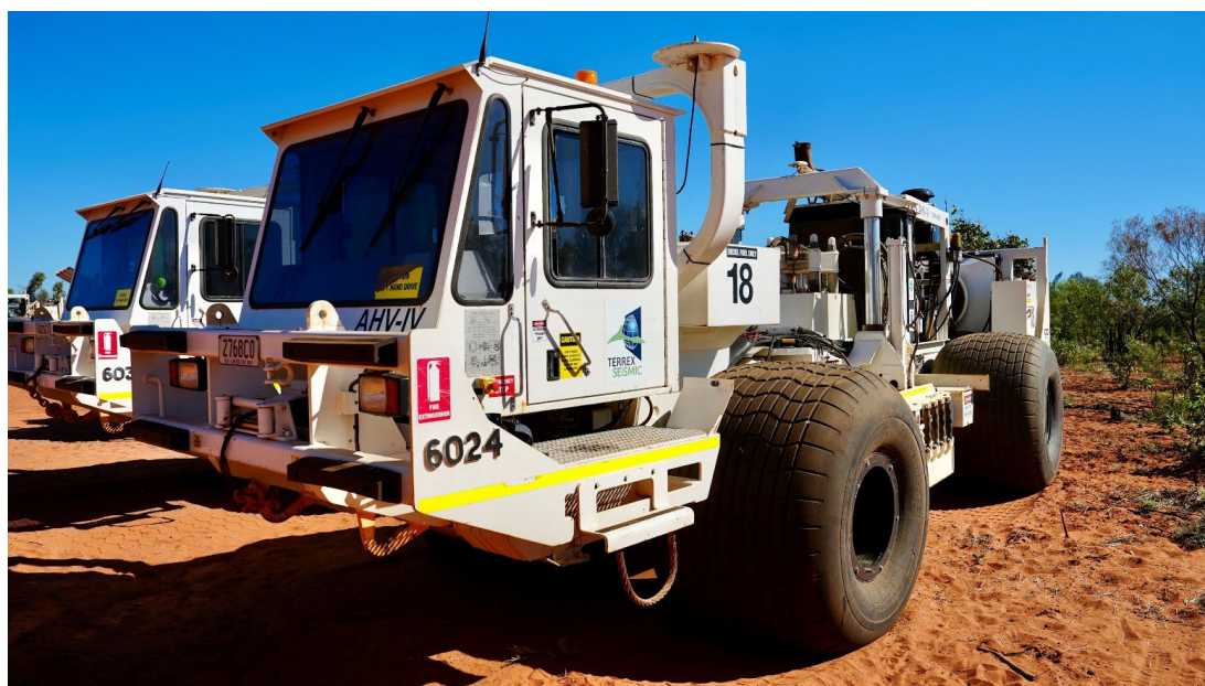
Terrex Vibroseis trucks on site
