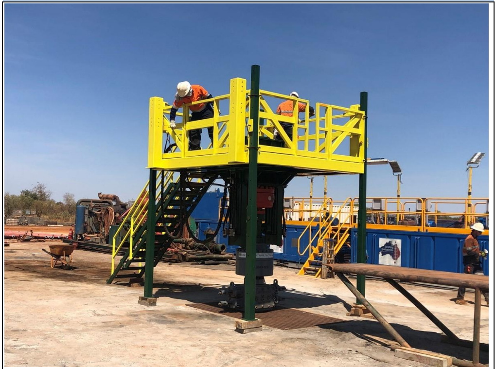
Fig. 3: BRU's Jacking Platform
