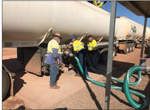
Wyndham Tank 10 unloading facility
