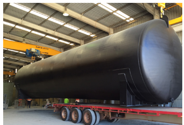
1,250 bbl storage tank under construction
