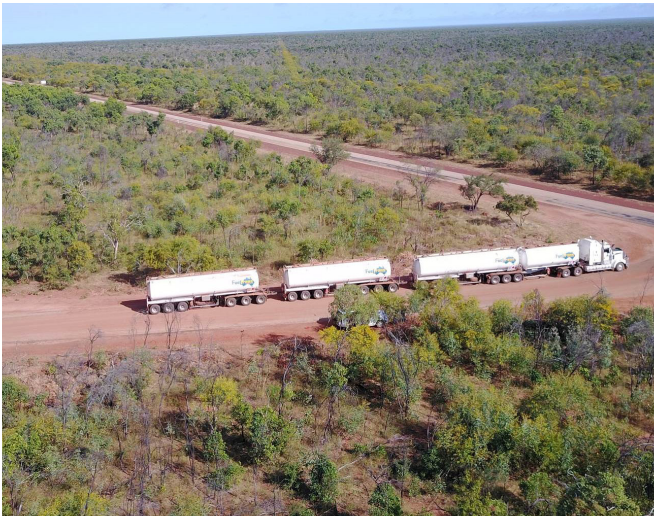
FTA quad road train with ~880 bbls of Ungani oil bound for Wyndham Port
