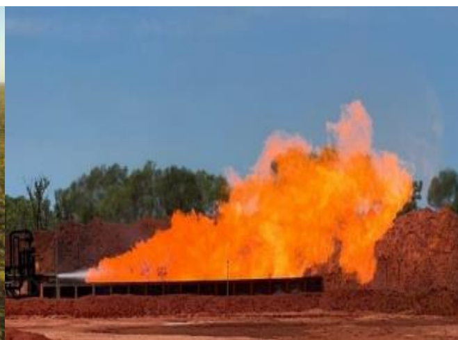
Figure 10: Rafael: Gas flow test
